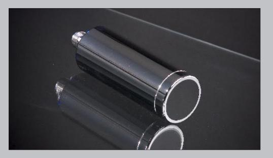
The Oceanscan Multi-Return Altimeter fulfills many of the sonar data capture requirements of the oceanographic and scientific communities. This unit differs from most Altimeters of the "first-return" type by digitising the receiver output at high speed into a FIFO memory. The range to the sea-bed is then calculated in the digital domain by the mathematical processing algorithm programmed into the internal RISC microcontroller.
